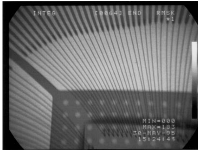
Fig. 2. X-ray micrograph of a molded package showing wire sweep. The curvature in the wire trajectories is induced by resin flow during soldering.
